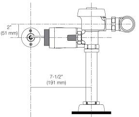
**2.** Drill two (2) mounting holes into wall and mount flange using the appropriate fasteners for the particular wall type.
